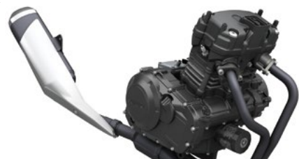
248cm 3 parallel-twin engine
